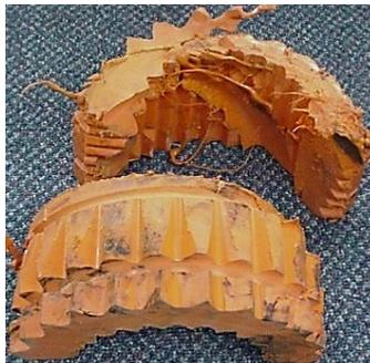
Figure 3 Failed Not Listed/Approved Fire Pump System Elastomeric Coupling
